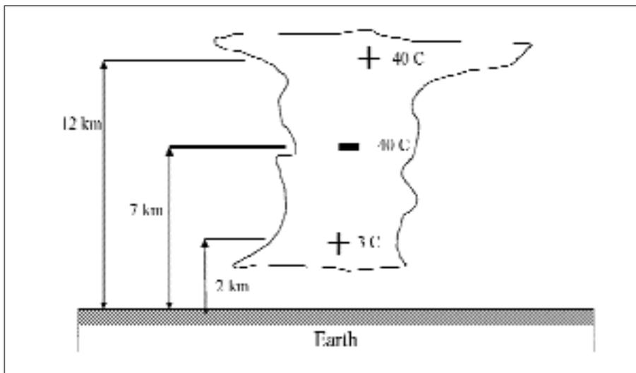
Figure 7. An idealized scheme of the electric charge distribution in a thundercloud according to the tripole model. Charge values and heights are roughly indicative of real values and they attempt to summarize the average situation reported by the various in situ measurements available in literature. Charge values are reported inside the cloud and they are expressed in Coulomb.
