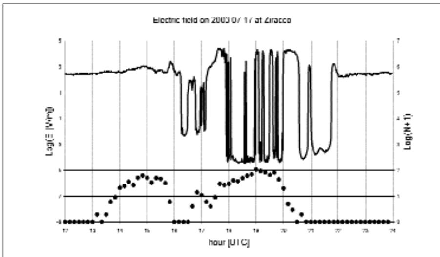
Figure 5. The stormy part of the Earth electric field recorded at Ziracco on 17 July 2003. The moving average over one minute of the electric field intensity has been plotted (solid line). The number of lightning strikes clustered every ten minutes over an area of  $2^\circ \times 2^\circ$  (about 35,000 km<sup>2</sup>) centered on the field mill position are reported as dots. The electric field is set positive when it is pointing downward and it is reported in black.
