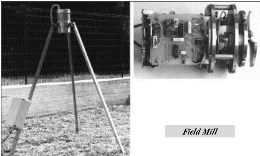
Figure 2. Pictures of the field mill. The mill is placed at 1 m above the ground and it is connected to a personal computer for ongoing data storage. Signals are sent to the computer through a coaxial wire.
