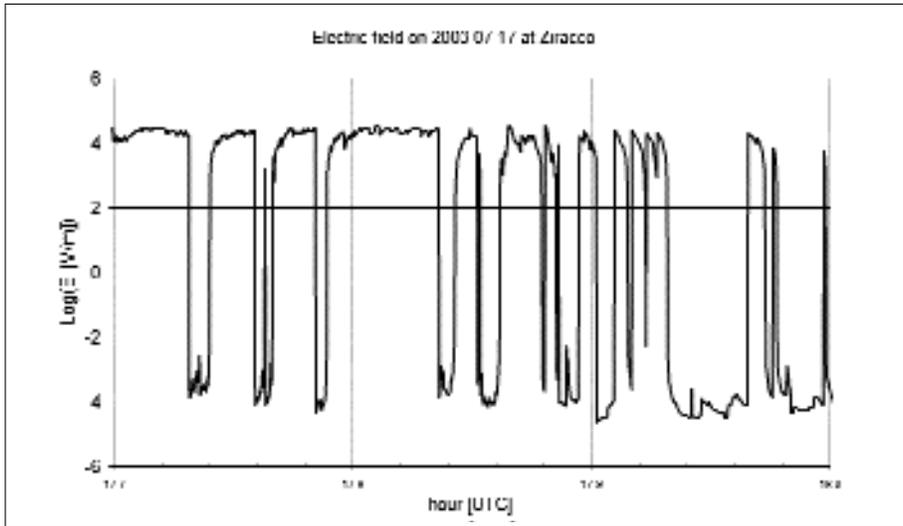
Figure 6. Zoom of the Earth electric field reported in figure 4. This part of the time series is dominated by the lightning discharges, which produce sudden inversions of the field with amplitudes of several kilovolts. The non-symmetric shape of the inversions is evident. In fact, each inversion has a sudden inversion followed by a slower recovery of the original field. The pattern is very similar to that of a capacitor that is discharged and then recharged.
