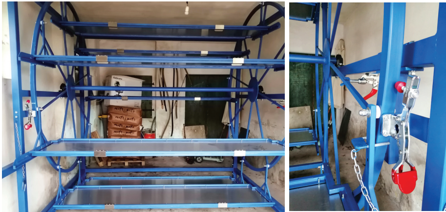
Figure 6(a) and 6(b) In red are the safety systems mounted on the machine: brakes, fork stops on the wheel and the box frame so that they do not wobble while working, and fork stops on the square spoke of the wheel to prevent it from moving while working on the box. Two hinges can be seen on the boxes to stop the bottom from sliding out.
