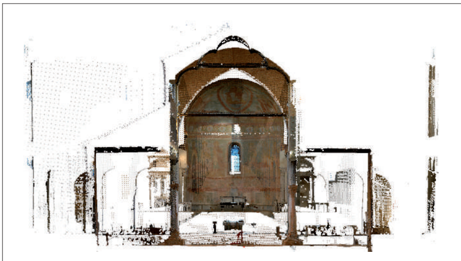
Figure 15. Prospet/sezion trasversâl de Basiliche cun viodude viers la abside. / Figure 15. Transversal section/prospect of the Basilica towards the apse.
