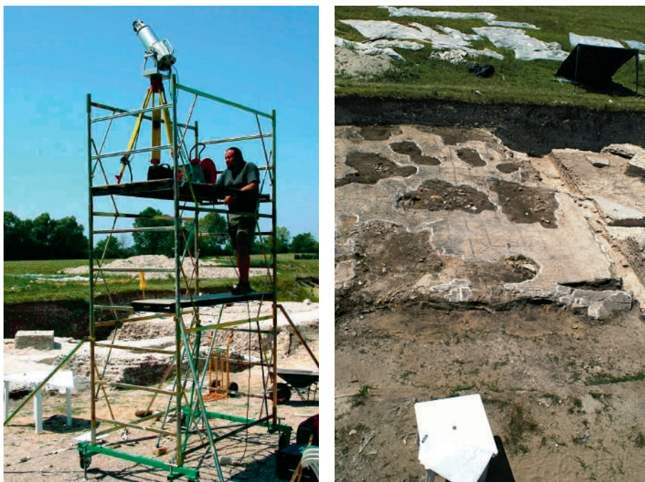
Figure 5. Acuisizion dai dâts midiant Riegl Z360I di une impalcadure inte aree sud des Termis Romanis (a çampe). Une imagjin digjitâl de “Aule Sud” çjapade sù cun la çjamare metriche Nikon D100 (a diestre). / Figure 5. Data acquisition with Riegl Z360I from a scaffold in the Roman Thermae southern area (left). One digital image of the “Aula Sud” so acquired with the Nikon D100 photogrammetric camera (right).
