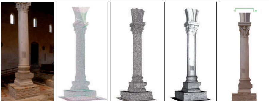
Figure 14. Une colone de Basiliche (a çampe): dal nûl di ponts TLS al prospet midiant ortofoto (a diestre). / Figure 14. One Basilica column (at left): from the cloud of points to the prospect by orthophoto (at right).
